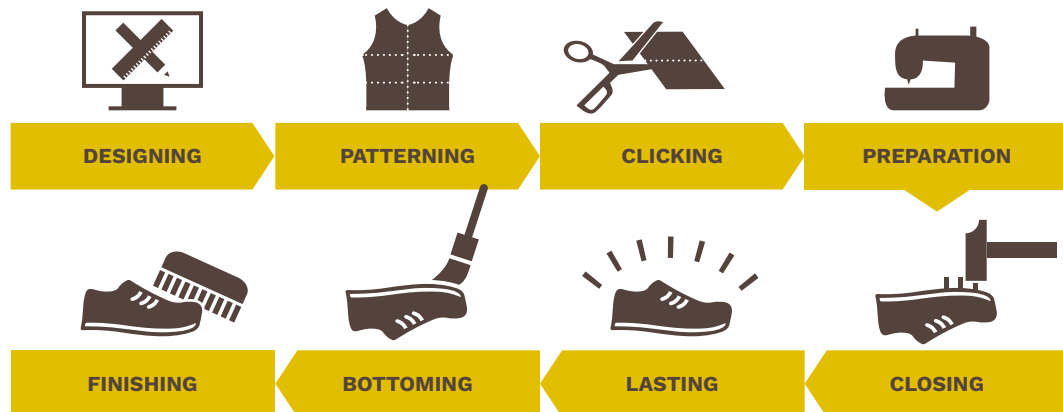
Figure 7. Processes of leather goods manufacturing (in this case footwear)
